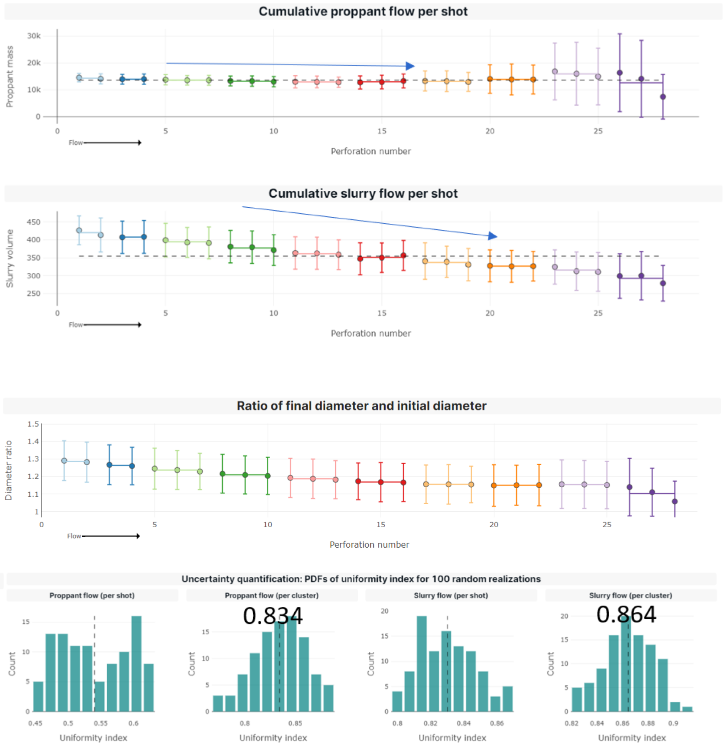
Figure 15—Results of the calibrated simulation model for Case Study 1. The ‘Ratio of final diameter and initial diameter’ plot is consistent with the observations shown in Figure 14. Dots correspond to individual shots, while horizontal lines correspond to the average for clusters.
